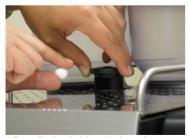
7. Open coffee chute that's located on the top of the machine, insert a cleaning tablet, then confirm by pressing the COFFEE CLEAN button. Coffee clean process will take approximately 20 minutes.
