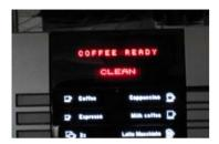
1. When machine Displays "Clean", a coffee clean must be performed.
